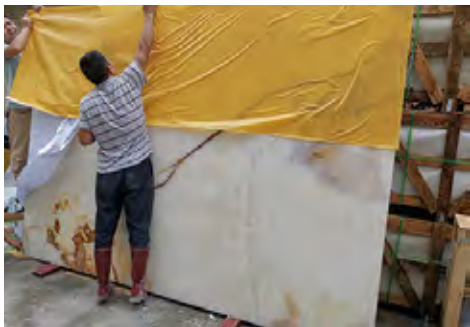
1. Covering the slabs by masking tap
