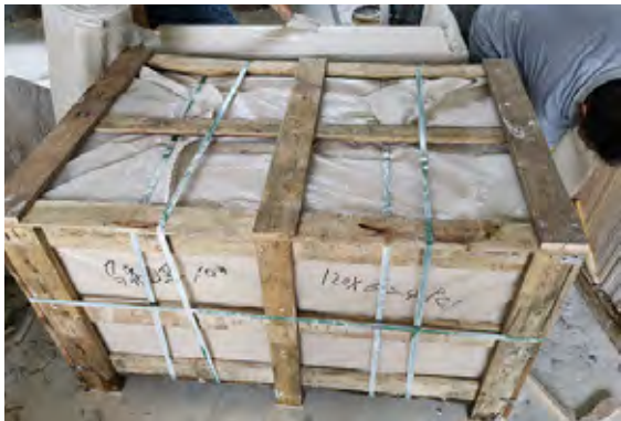
5. Nailing the cover and having a belt packing
